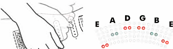
Strum your guitar. Strings that are in tune will be represented by two green LEDs. Strings that need tuning are represented by two red LEDs below (flat) or above (sharp) the middle row.
