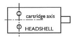
Align the cartridge carefully so it lies at right angles to the fixing screw holes. If the headshell sides are parallel they can be used as a reference.
