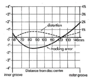
The tracking error of an arm as it crosses an LP produces distortion, shown here. Careful alignment of cartridge in the headshell and of arm geometry minimises the problem
