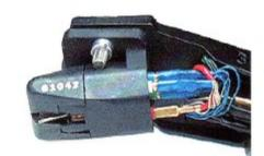
Shown left - the edge of the cartridge must align perfectly with the headshell reference face to minimise distortion from tracking error
